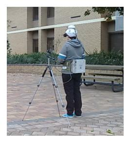
Figure 1: The setup of the augmented viewport technique with a zoom lens camera mounted on a tripod next to the user
